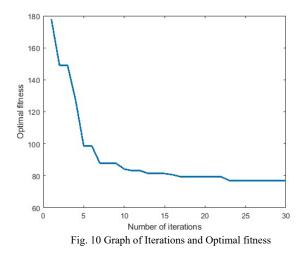
As shown in Figure 10, the whole algorithm has a fast iteration speed. When it iterates to 20 times, it is basically close to the optimal fitness. This advantage will bring great convenience for the algorithm to be used in the real underwater environment.
